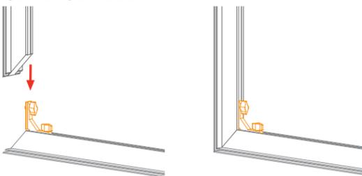
Keep corner connectors attached to horizontal extrusions.
