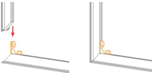
Keep corner connectors attached to horizontal extrusions.
